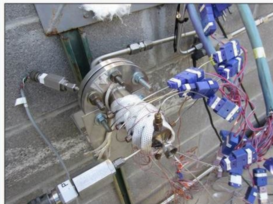
(15) E-type thermocouples, (3) 500 psi pressure transducers, (1) turbine flow meter were used to capture test data
