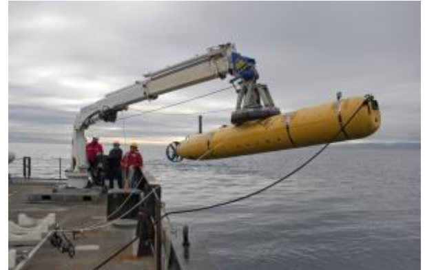
The Dorado Gulper AUV being deployed from R/V Rachel Carson. Image Credit: MBARI
