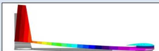
Above: FEM with component close-up view and wing deflection deformation and contour Left: FEM Right wing force loading (top) and FEM with boom deflection deformation and contour (bottom)
